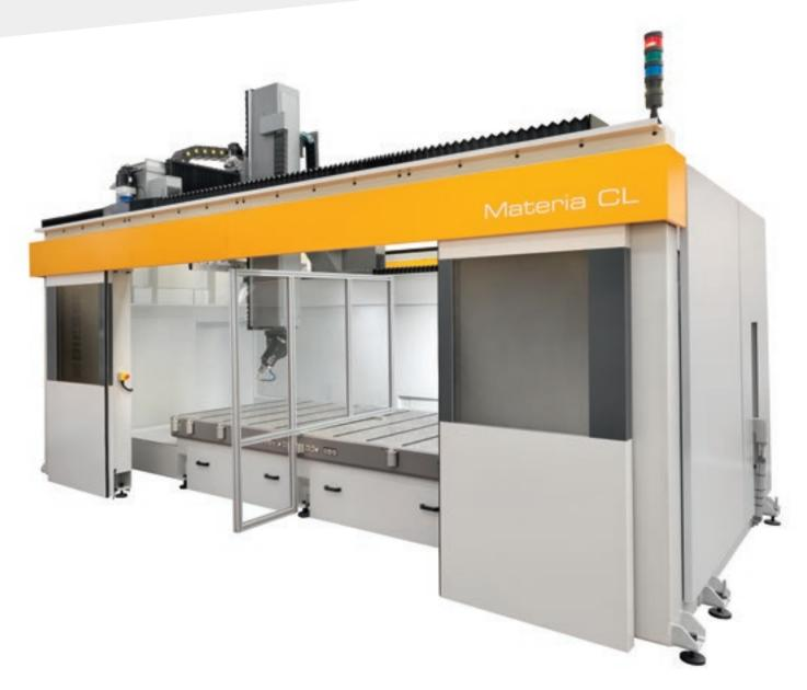
A removable partition can be installed in the working area to permit pendular machining.
