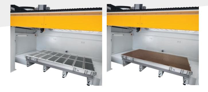
The grid surface allows the operator to insert the gasket in any configuration, creating a specific vacuum area. An internal chamber ensures the even distribution of the vacuum all over the work table. Each area is controlled by a piece locking button, an area selection button, and a start button.
